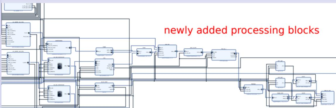
Dual PRN generator and cross-correlation with the received datastream frequency transposed using the NCO.
