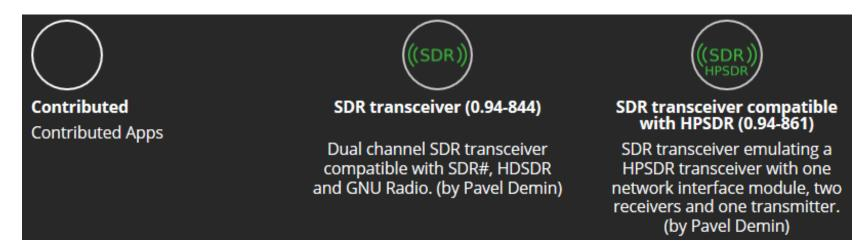
These applications configure FPGA and start TCP or UDP servers that communicate with SDR programs running on a remote PC:
