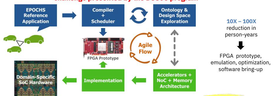
**Agile methodology** to quickly design and implement an **easily programmed** domain-specific SoC for real-time cognitive decision engines in connected vehicles **"Super"-Domain:** Software-Defined Radio + Computer Vision
