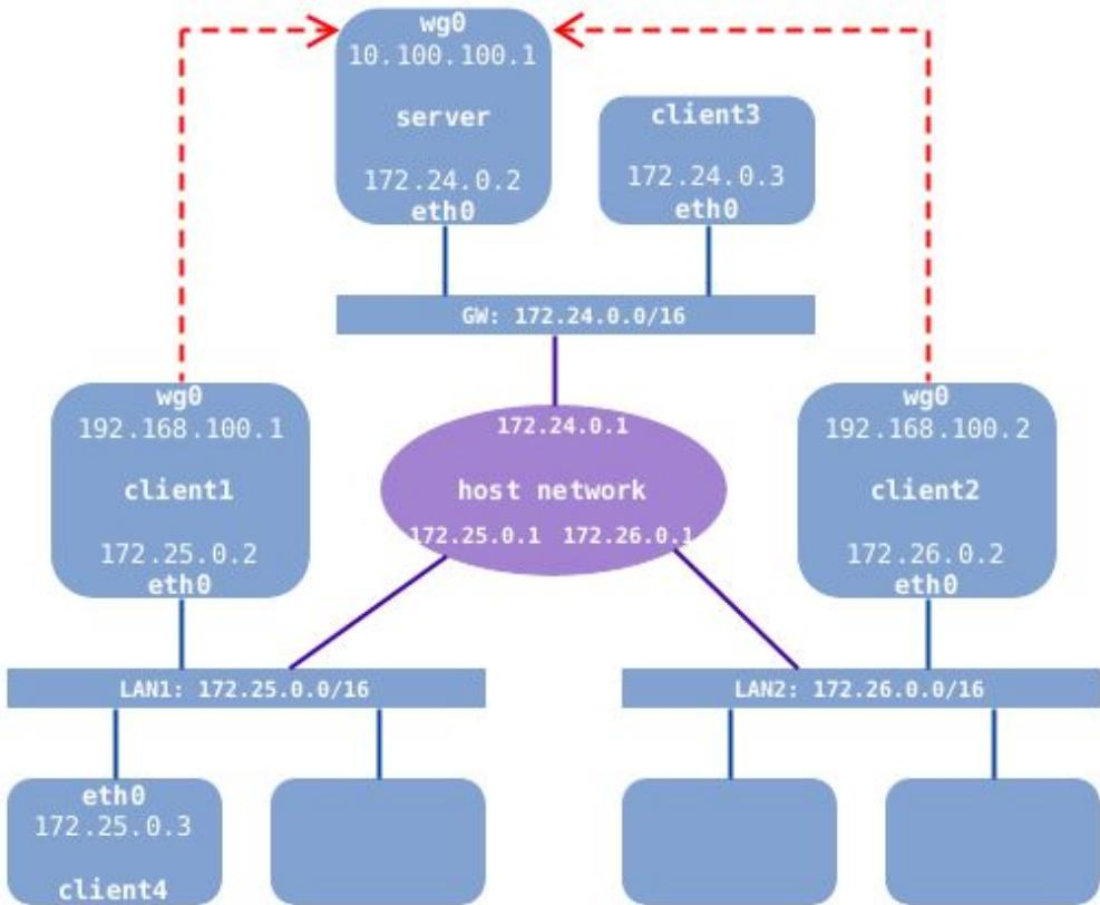
This test is related to Usecase #4, where a containerized application on the cloud, which is located on the same docker network as the WG server, can access clients that don't have a public IP. At the same time, clients can access the application, but not each-other.
