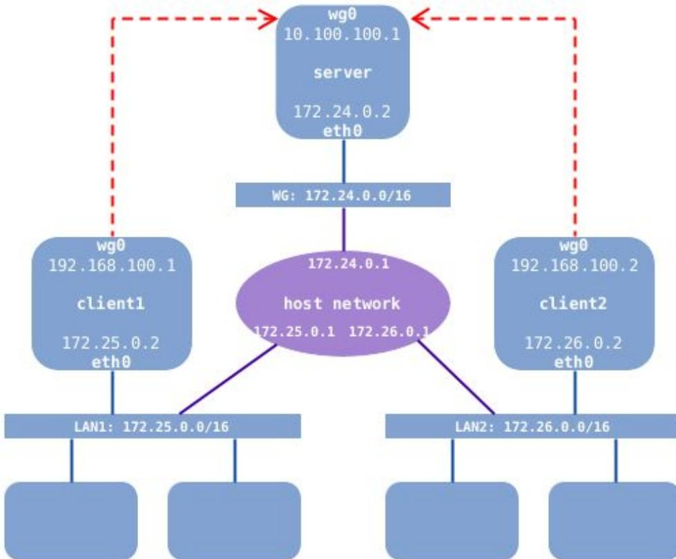
This test is related to the Usecase #2, where clients can access each-other, but cannot access the internet through the WG interface (because of the setting **ALLOW\_INTERNET\_ACCESS=no**).
