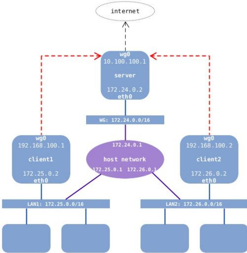
This test is related to a customized version of Usecase #1, where WG clients can also ping each-other, besides accessing the internet through the WG server. This requires the setting **CLIENT\_TO\_CLIENT=yes** (enabled).
