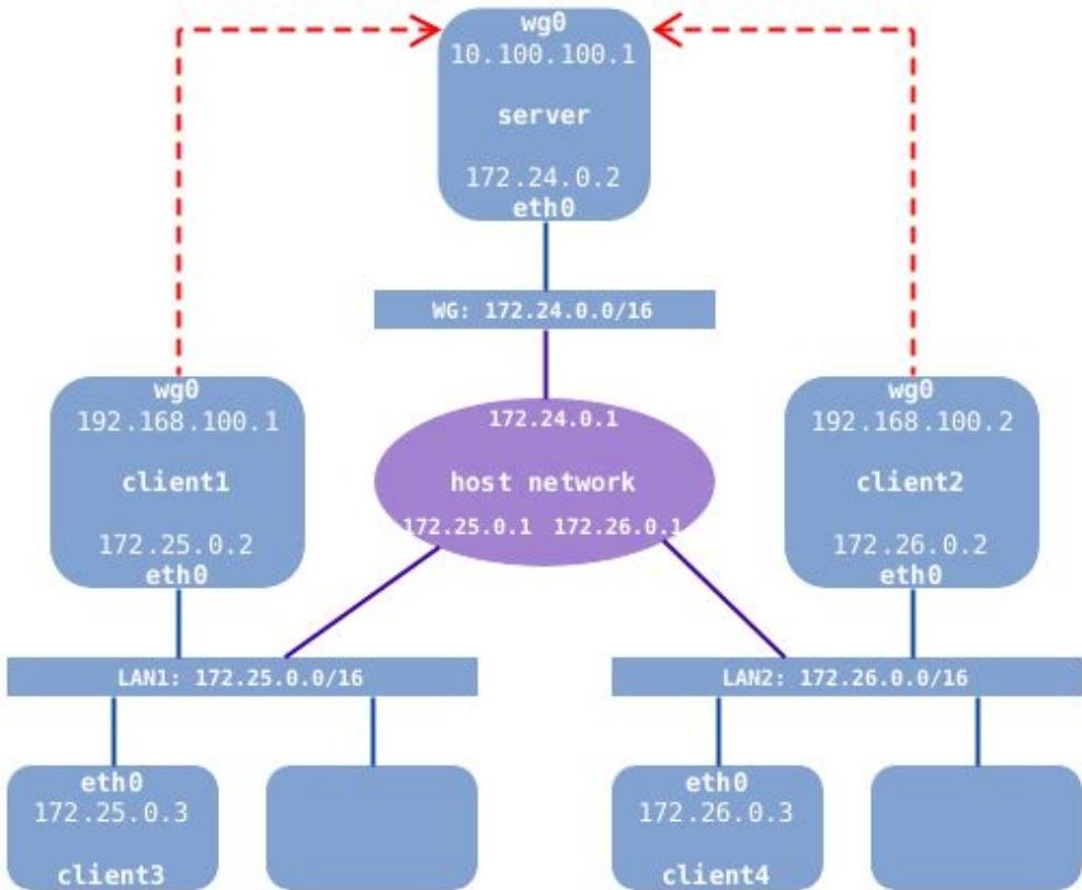
This test is related to the Usecase #3, where clients on two different private LANs, can access each-other through the WG network.
