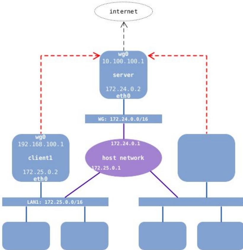
The first test is related to the Usecase #1, where a WG client can access the internet through a secure connection to the WG server.
