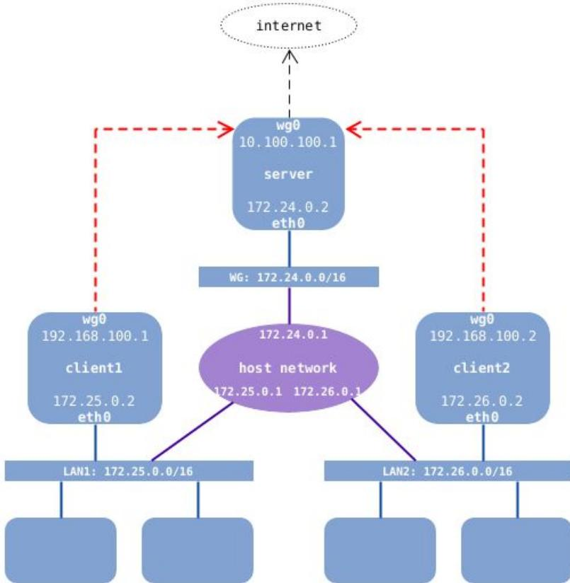
This test is related to the Usecase #1, where a WG client can access the internet through a secure connection to the WG server. By default, two different clients cannot ping each-other. The setting **CLIENT\_TO\_CLIENT** by default is commented out (which means disabled).
