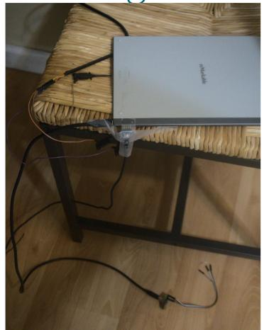
The pogo pins provide UART TX and debug downloader mode (with uuu)
