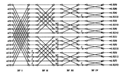
Figure 3: Radix-2<sup>2</sup> DIF FFT flow graph for N = 16
