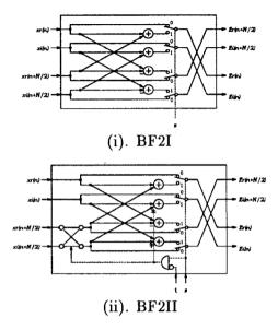
Figure 5: Butterfly structure for R2<sup>2</sup>SDF FFT processor
