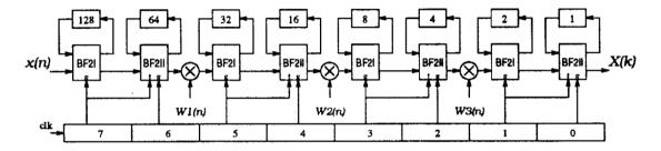
Figure 4: R2<sup>2</sup>SDF pipeline FFT architecture for N = 256
