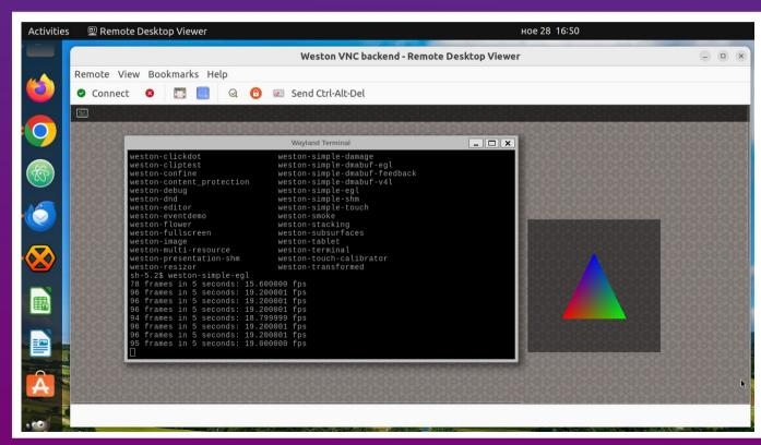
With VNC enabled weston-simple-egl runs with up to 20fps on Raspberry Pi 5
