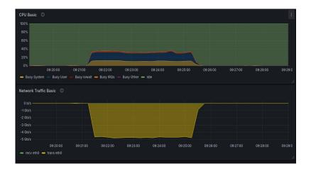
~ 0.7 CPU core when saturating network on Get
