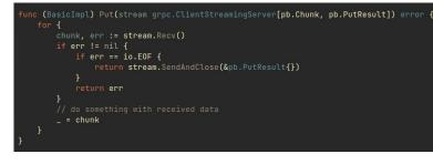
/ Recv reads one message from the stream of responses generated by the serve / The type of the message returned is determined by the Res type parameter / of the GenericClientStream receiver.
