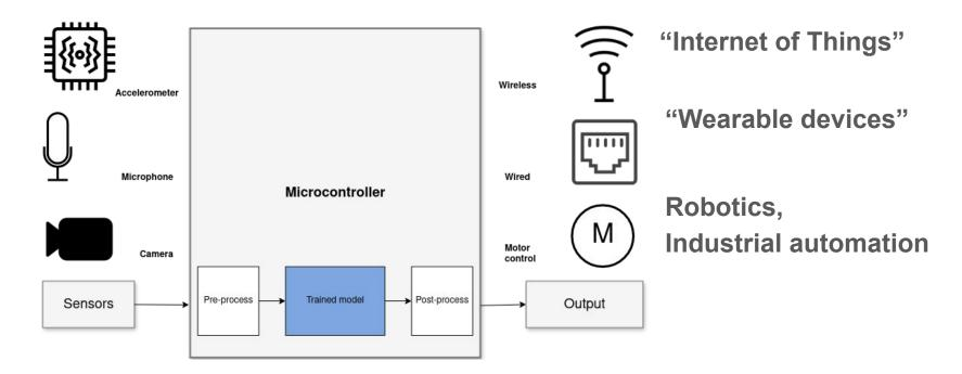
1) Read sensors -> 2) Process data \* -> 3) Transmit/act on data data
