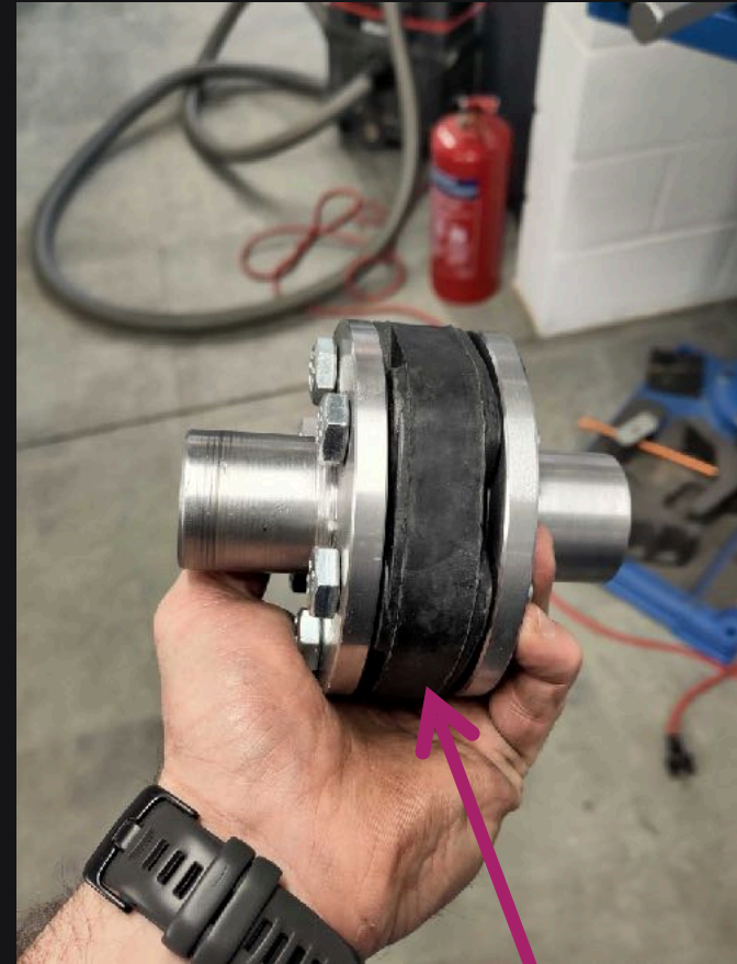
Custom junction piece to connect the motor to the gearbox
