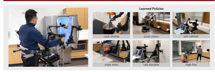
**Figure 1:** *Mobile ALOHA* > . We introduce a low-cost mobile manipulation system that is bimanual and supports whole-body teleoperation. The system costs \$32k including onboard power and compute. *Left:* A user teleoperates to obtain food from the fridge. *Right: Mobile ALOHA* can perform complex long-horizon tasks with imitation learning.
