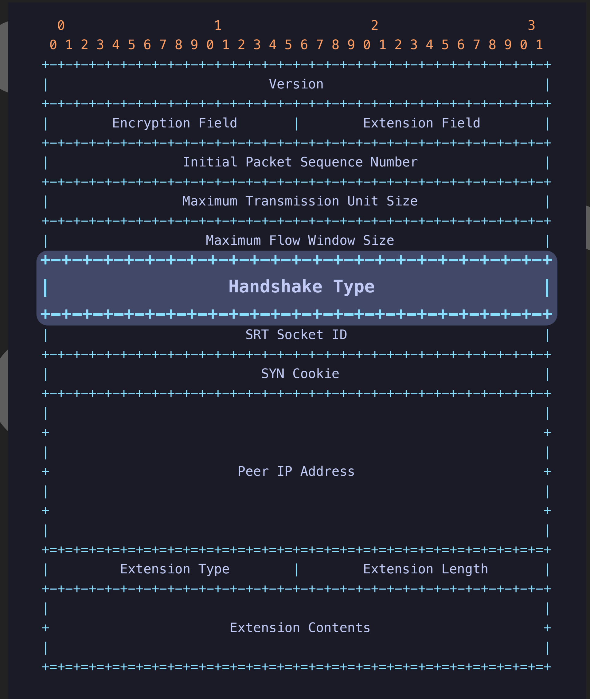
SRT Handshake packet structure
