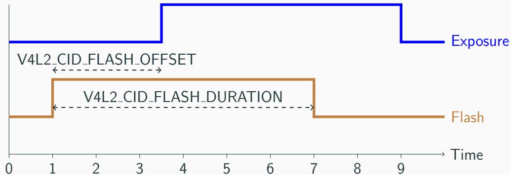
Figure 4: V4L2 flash duration and offset CID timing
